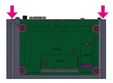
2. Locate the mini-PCIe slot on the mainboard and install the Wi-Fi or LTE module into the slot. Then secure the module with a screw.
