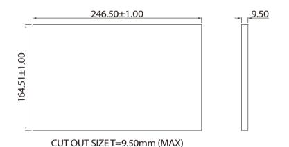
3. Slide the panel PC through the hole until it is properly fitted against the panel.
