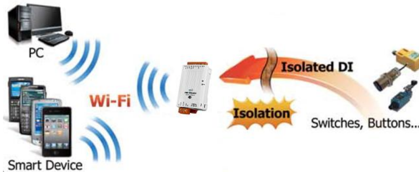
Figure 4-1: tWF + PC/Laptop/Smart Device application architecture
