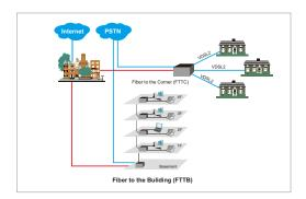
The VDSL2 technology is also deployed at the last mile of internet access. The ISP uses the fiber cable as backbone uplink to the basement of building (FTTB) or corner of streets (FTTC) and uses the existing 1 pair twisted cable of POTS system to carry voice and Ethernet data stream to users via VDSL2 signal.
