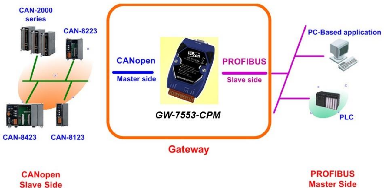
Figure 1 Application architecture of the GW-7553-CPM module
