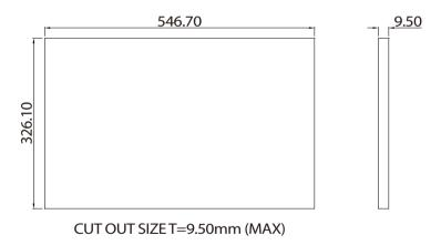
3. Slide the panel PC through the hole until it is properly fitted against the panel.
