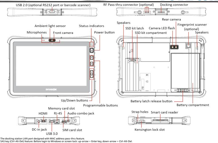
SAS key (Ctrl-Alt-Del) feature: Before login to Windows or screen lock: up-arrow = Enter key, down-arrow = Ctrl-Alt-Del. In Windows: up-arrow and down-arrow = volume or brightness adjust, depending on the setting in BIOS or Quick Menu.
