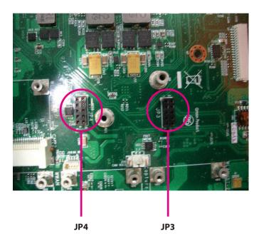
2. Connect the OBDII module to JP4 and JP3 and secure the OBDII module with screws.
