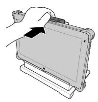
3. Ensure the R11L tablet PC is tightly secured to the docking cradle.
