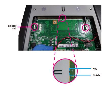
3. Insert the module into the socket at an approximately 30 degree angle. Apply firm even pressure to each end of the module until it slips down into the socket. The contact fingers on the edge of the module will almost completely disappear inside the socket.
