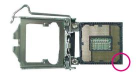
The CPU's notch will at the same time fit into the socket's alignment key.
