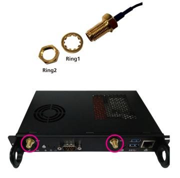
6. Connect the external antennas to the Wi-Fi antenna jacks.
