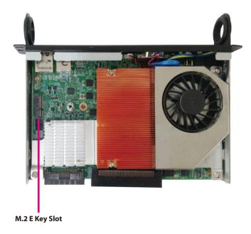
2. Insert the Wi-Fi module into the M.2 E key slot at a 45 degree angle until the gold-plated connector on the edge of the module completely disappears inside the slot.
